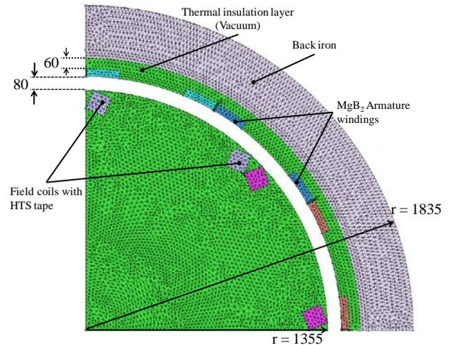
Fig. 2. 2D FEM analysis model for 8-pole fully superconducting wind turbine generator (1/4 model, unit: mm).
