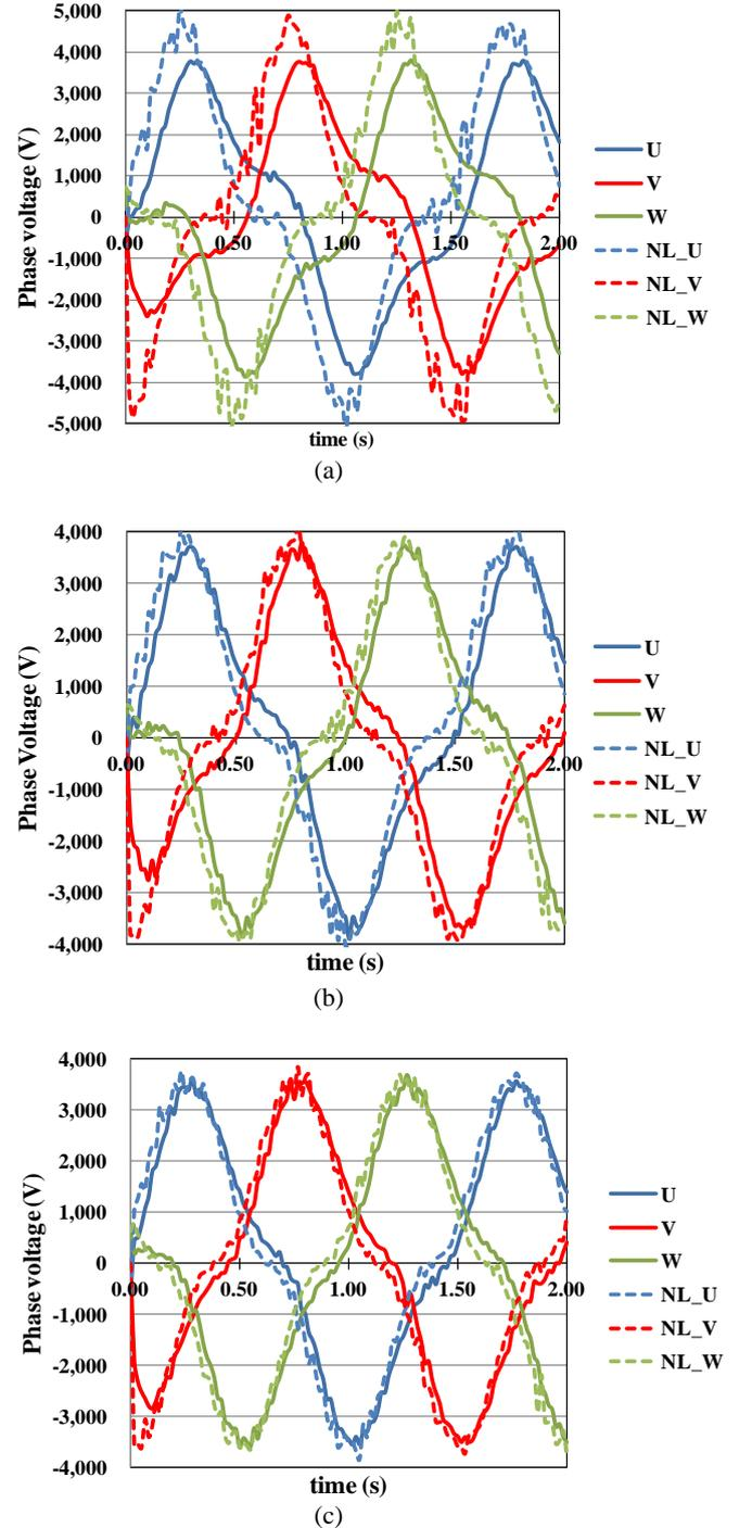
Fig. 3. Phase voltage waveforms of three generators. (a) - (c) represents generator A, B, and C respectively. "NL" in graphs means "No Load".
