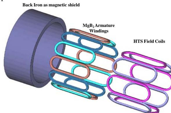
Fig. 1. Illustration of fully superconducting wind turbine generator.
