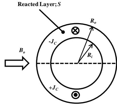
Fig. 6. Cross section of a fully penetrated MgB<sub>2</sub> filament by applied magnetic field;  $B_o$ .
