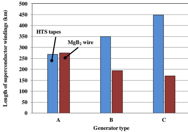
Fig. 5. Total length of two superconductor windings for three kinds of generators.
