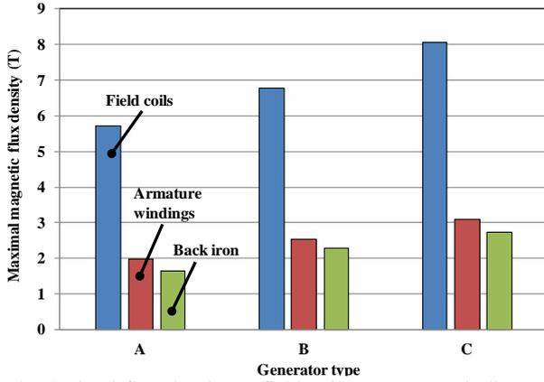
Fig. 4. Maximal flux density at field coils, armature windings, and back irons.
