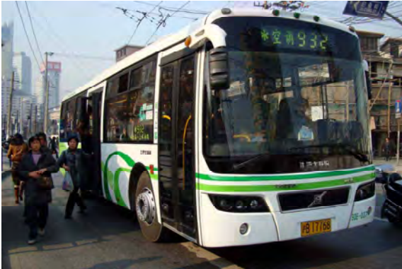
Fig. 4. Capacitor-operated Bus in Shanghai.
