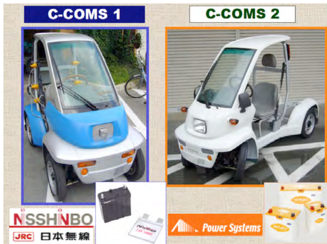
Fig. 2. C-COMS Driven Only by Supercapacitors.
