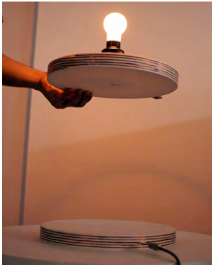
Fig. 12. Experiment of Wireless Power Transfer at Hori Lab.
