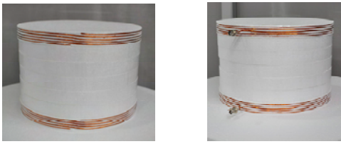
(a) Open end and opposite of feeding point. (b) Open end and feeding point.
