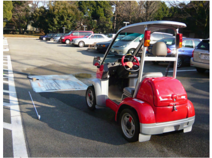
Fig. 11. Setting of slippery road experiment.
