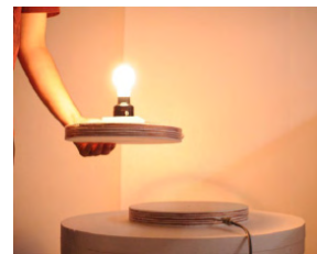
Fig 9. The transmitting and receiving antenna used to transmit power to light up a 40W bulb.
