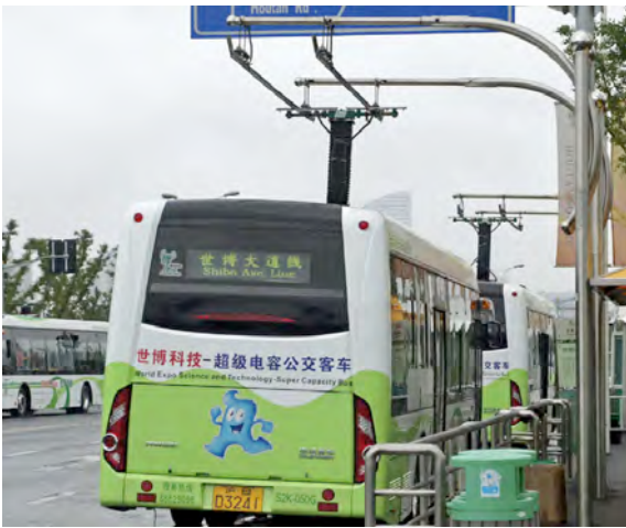
Fig. 5. Illustration of Charging an EV at a Bus-stop. (Charging Duration: less than 30 s)
