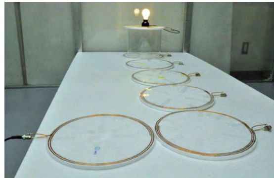
Fig. 3. Transfer distance extension using repeating antennas.
