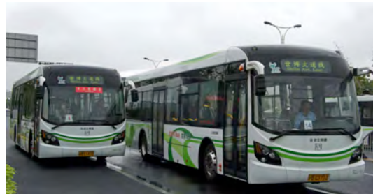
App. Fig. 1. Capacitor bus (left) and battery bus (right) at Shanghai Expo.
