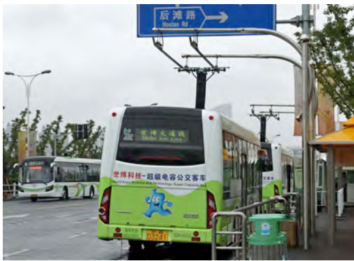
App. Fig. 3. Illustration of charging an EV at a bus stop. (Charging duration: less than 30 s)
