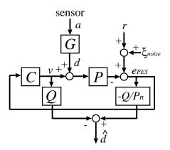
Fig.2: Block Diagram of Disturbance Observer to Estimate Disturbance
