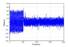
Fig.4: Time Series of PES under 100[Hz] vibration
