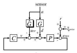
Fig.1: Block Diagram of Disturbance Rejection Control with Feedforward Input
