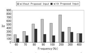
Fig.6: Comparison of  $3\sigma$  of Position Error Signal with/without Proposed Feedforward Input
