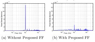
Fig.5: Characteristics of Fourier Transform about PES under  $100[\mathbf{Hz}]$  vibration
