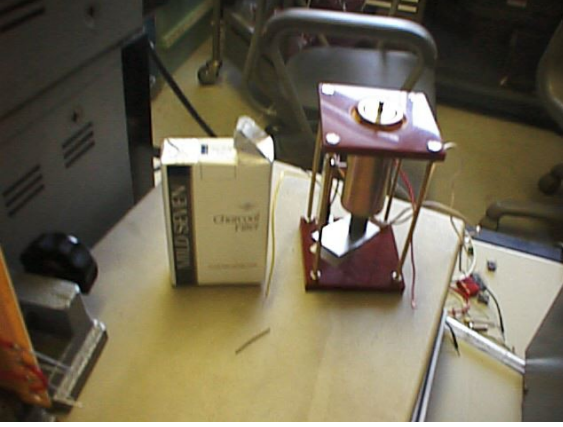
Fig.3: The real world actuator module consists of solenoid plunger.
