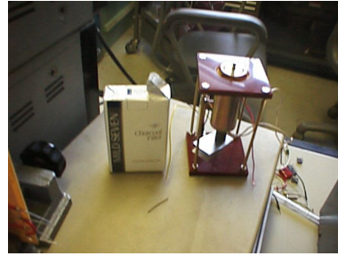
Fig. 5. The real world actuator module consisting of solenoid plunger. We can easily see attached position sensor. This position sensor is putted to use position signal in feedback controller.
