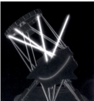
Fig. 3: Overview (2) of astronomical telescope "subaru". It is difficult to condense the ray of light because of distortion of the mirror by self weight.
