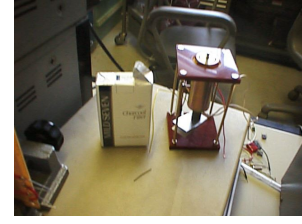
Fig. 4: The real world actuator module consisting of solenoid plunger. We can easily see attached position sensor. This position sensor is putted to use position signal in feedback controller.
