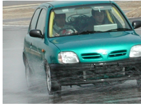
Fig. 13: Photo of turning experiments with 4W-motored EV “UOT Electric March II” (Fig. 14-15).
