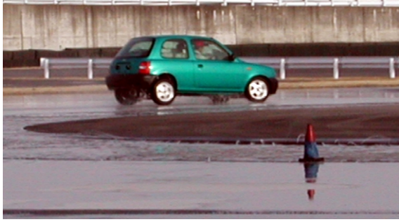
Fig. 13: Photo of turning experiments with 4W-motored EV “UOT Electric March II” (Fig. 14-15).
