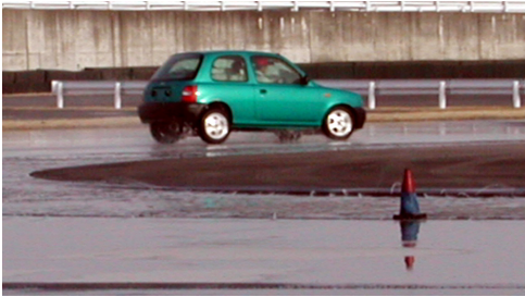
Figure 11: Photo of turning experiments with 4W-motored EV “UOT Electric March II”
