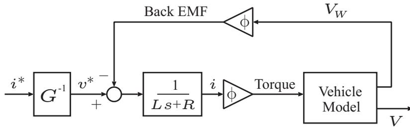
(a) The block diagram of the EV system installed separately wound DC motor with FF current control.
