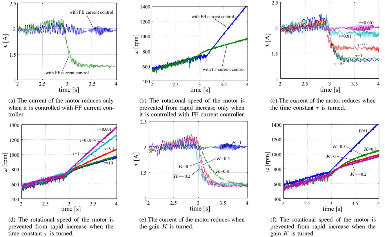
Fig. 8. The experimental results of the skid phenomenon with utilizing MG setup. (The torque (current) reduction characteristics can be confirmed. The current command  $i^* = 2[\text{A}]$ , the motor skids at about  $t = 3[\text{s}]$ .)
