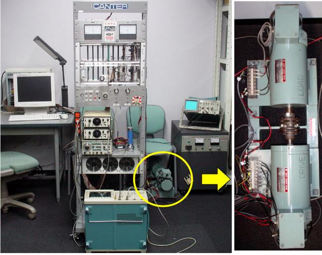
Fig. 6. Motor-Generator setup.
