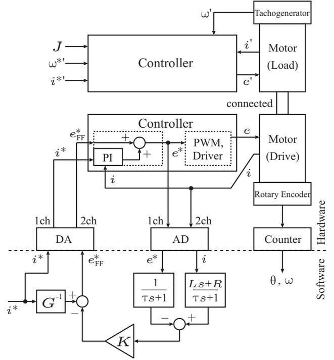
Fig. 7. The block diagram of the control system of MG setup. (The PI controller is not utilized when the FF current controller is utilized.)
