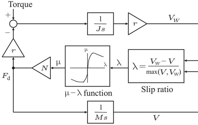
Fig. 2. The block diagram of the one-wheel vehicle model.
