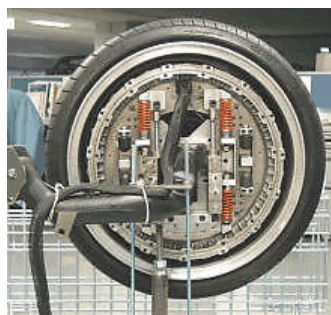
(a) Bridgestone Dynamic-Damper type In-wheel Motor System
