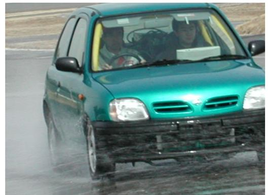
Figure 4: Photo of turning experiments with 4W-motored EV “UOT Electric March II” (Fig. 12-13).
