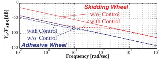
Figure 16: Bode diagram of  $H(s)P(s)$ .
