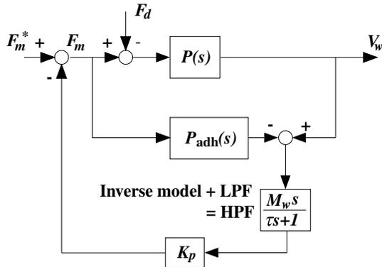
Figure 4: Block Diagram of wheel velocity controller.
