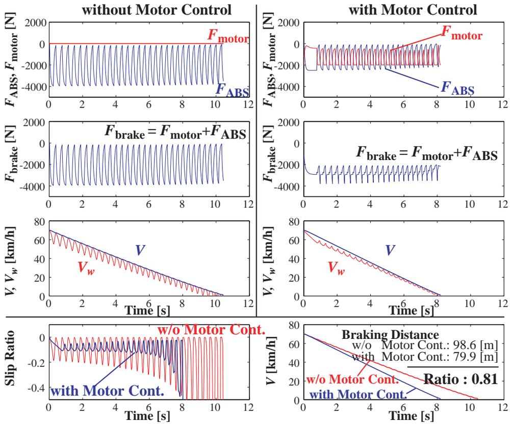
Figure 18: Simulation results with slippery road. ( $F_{\text{motor}}^* = -1500$  [N])
