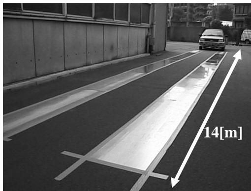
Figure 6: Test low- $\mu$  road for experiments.
