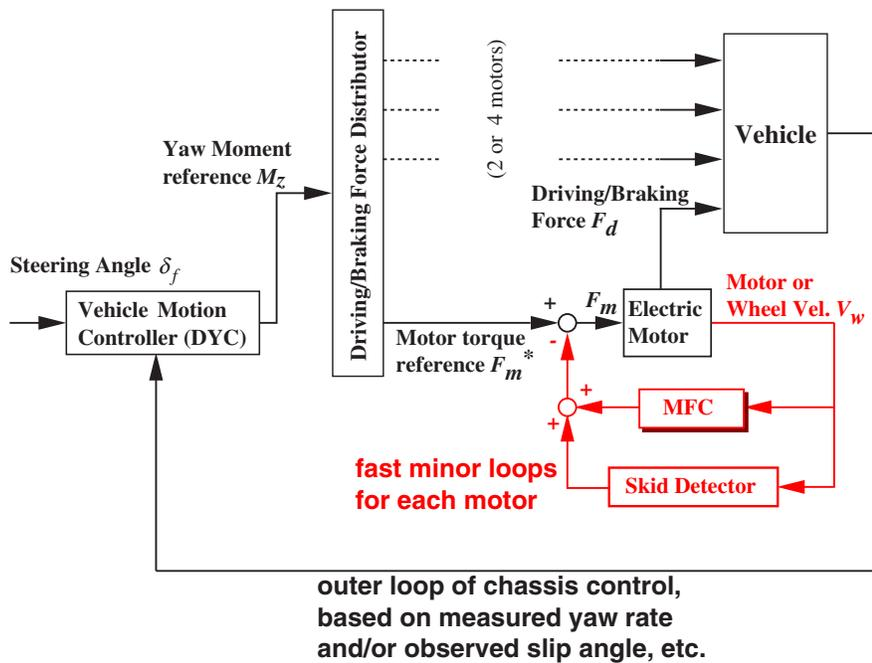
Figure 19: Our concept: minor-loop controller for each wheel.
