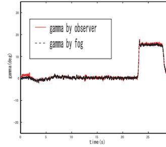
(b) Measured value and observer's output of  $\gamma$
