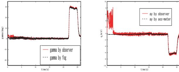
(b) Measured value and observer's output of  $\gamma$
