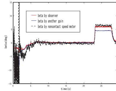
Fig. 8. No.4; Measured value and estimation of  $\beta$  with two different gain matrixes; Speed is 40km/h and steering angle  $\delta$  is 90[deg] when observer model has error
