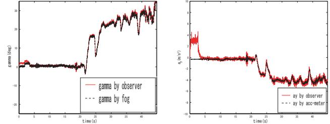
(b) Measured value and observer's output of  $\gamma$
