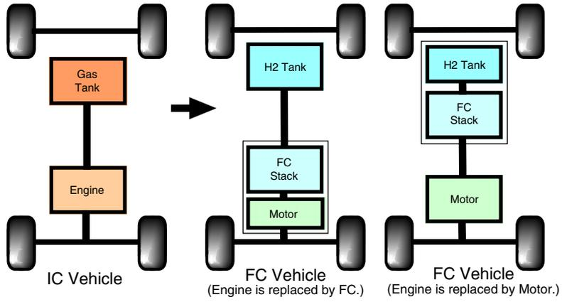
Fig. 29. Two ways to understand FCV.
