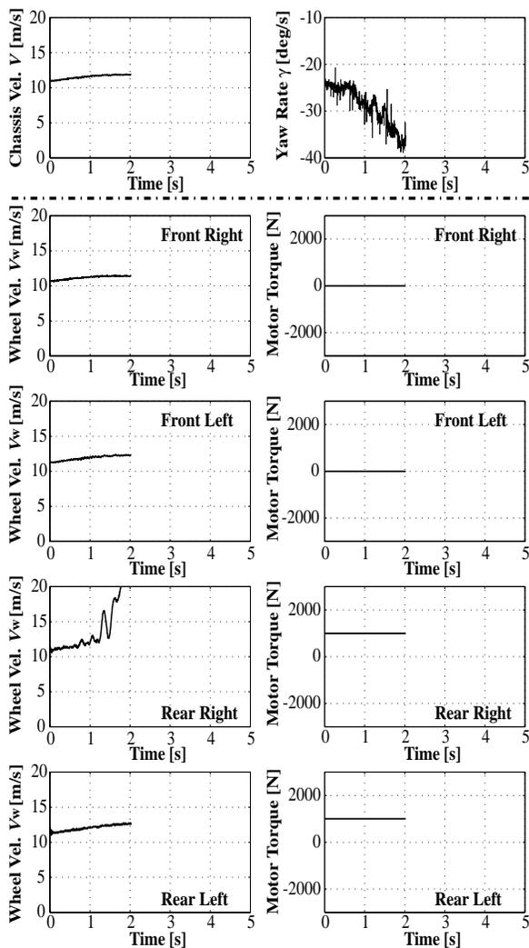
Fig. 18. Unstable cornering with sudden acceleration without MFC.
