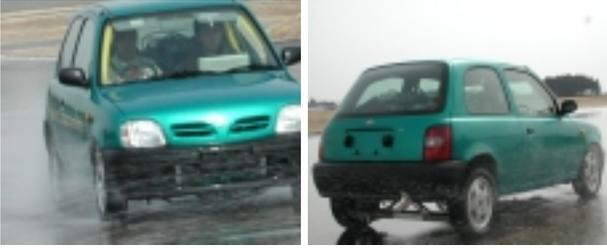
Fig. 13. Braking experiment of “UOT Electric March II”.
