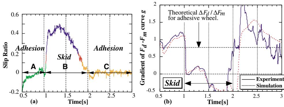
**Fig. 23. Experimental results of wheel skid detector.**
