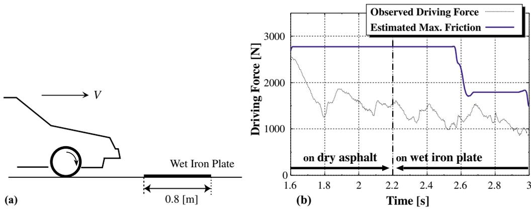
**Fig. 22. Experimental results of road condition estimator.**
