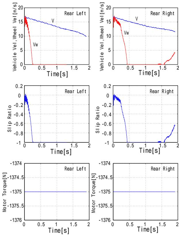
Fig. 10. Wheel lock in rapid braking “without MFC”.
