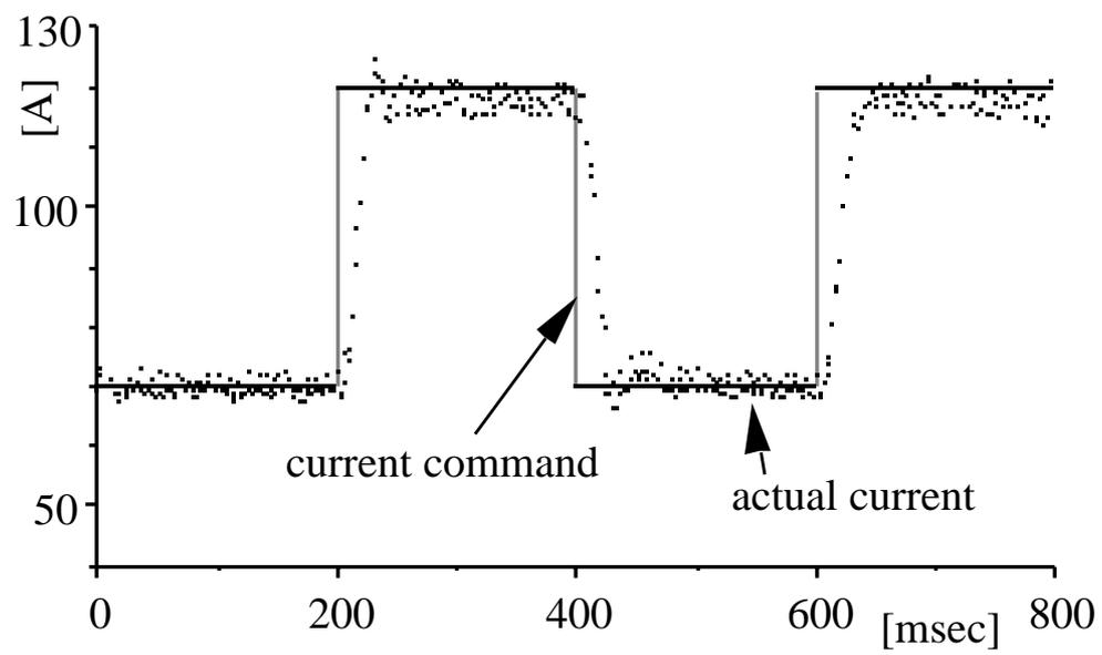
Fig.A-3. Basic experiment on the current response.
