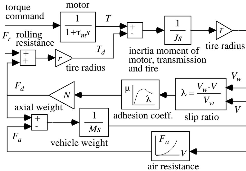
Fig.10. Vehicle model used in the simulation.
