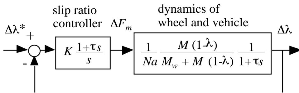
Fig.7. Slip ratio controller.
