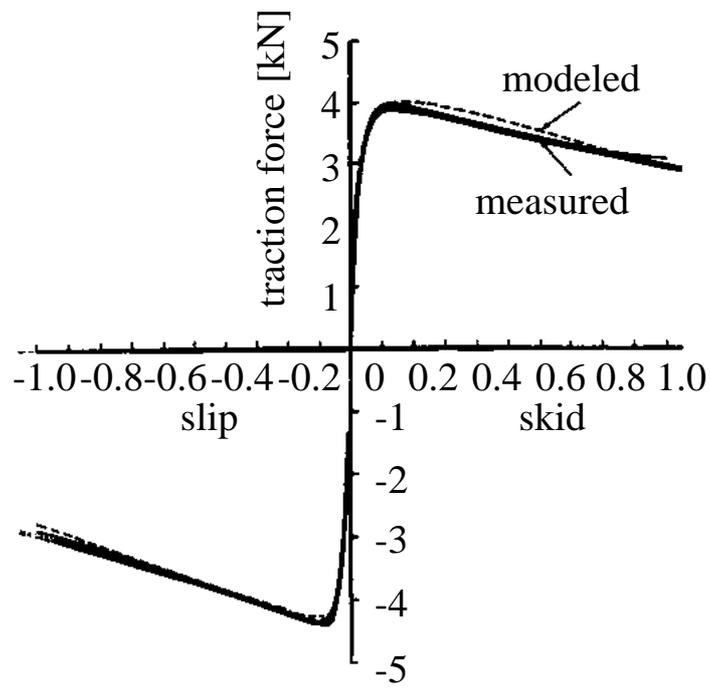
Fig.11.  $\mu$ - $\lambda$  characteristics used in the simulation.
