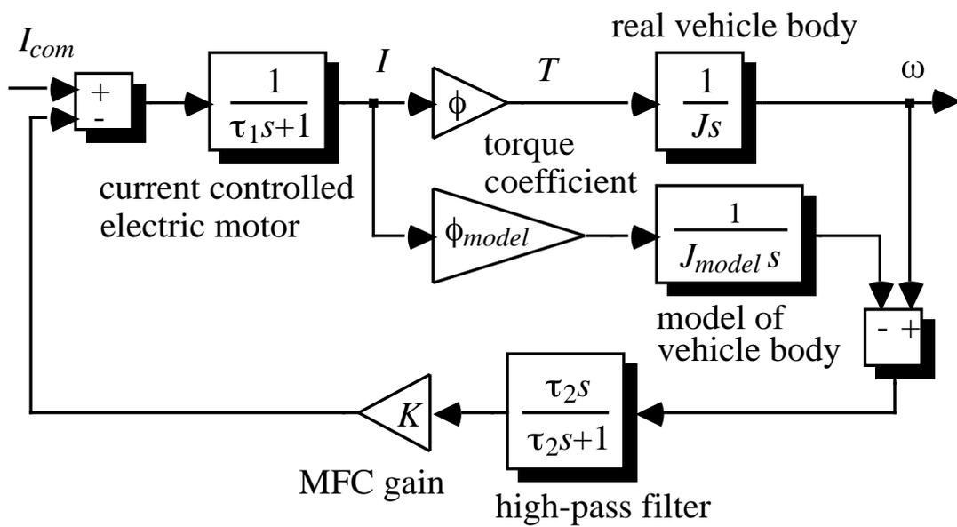
Fig.2. Block diagram of MFC.
