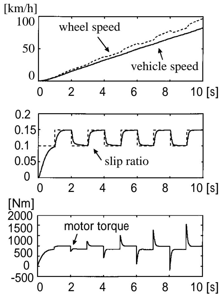
Fig.12. Simulation of the slip ratio control.
