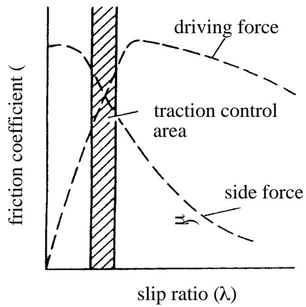
Fig.1. Characteristics of driving and lateral forces.
