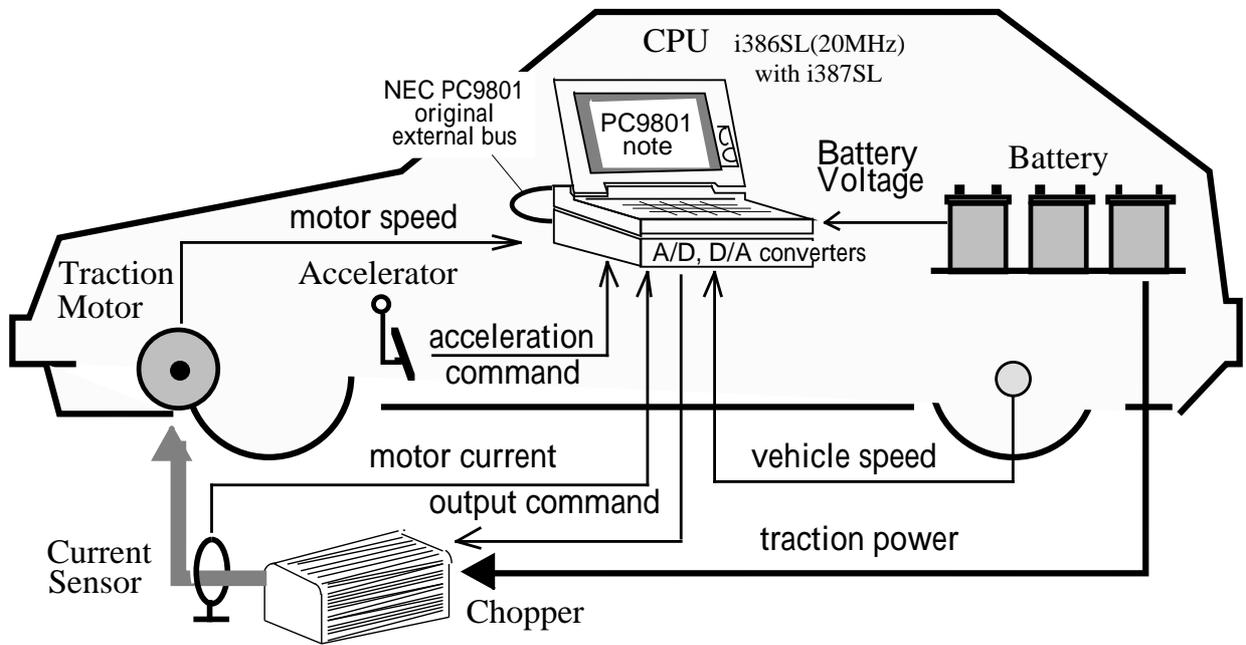
Fig.A-2. Configuration of UOT Electric March.
