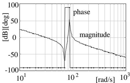
Fig.5 Frequency characteristics from  $\omega_M$  to  $T_M$ .
