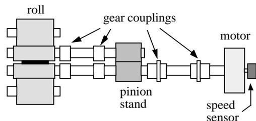
Fig.1 Illustration of the Steel Rolling Mill System.
