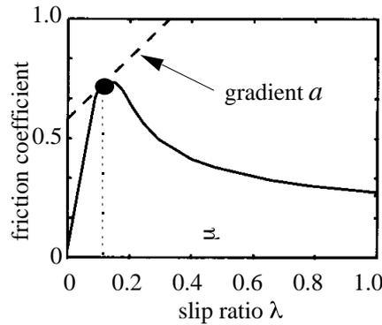
Fig.8. Nominal slip ratio is given by  $a=1$ .
