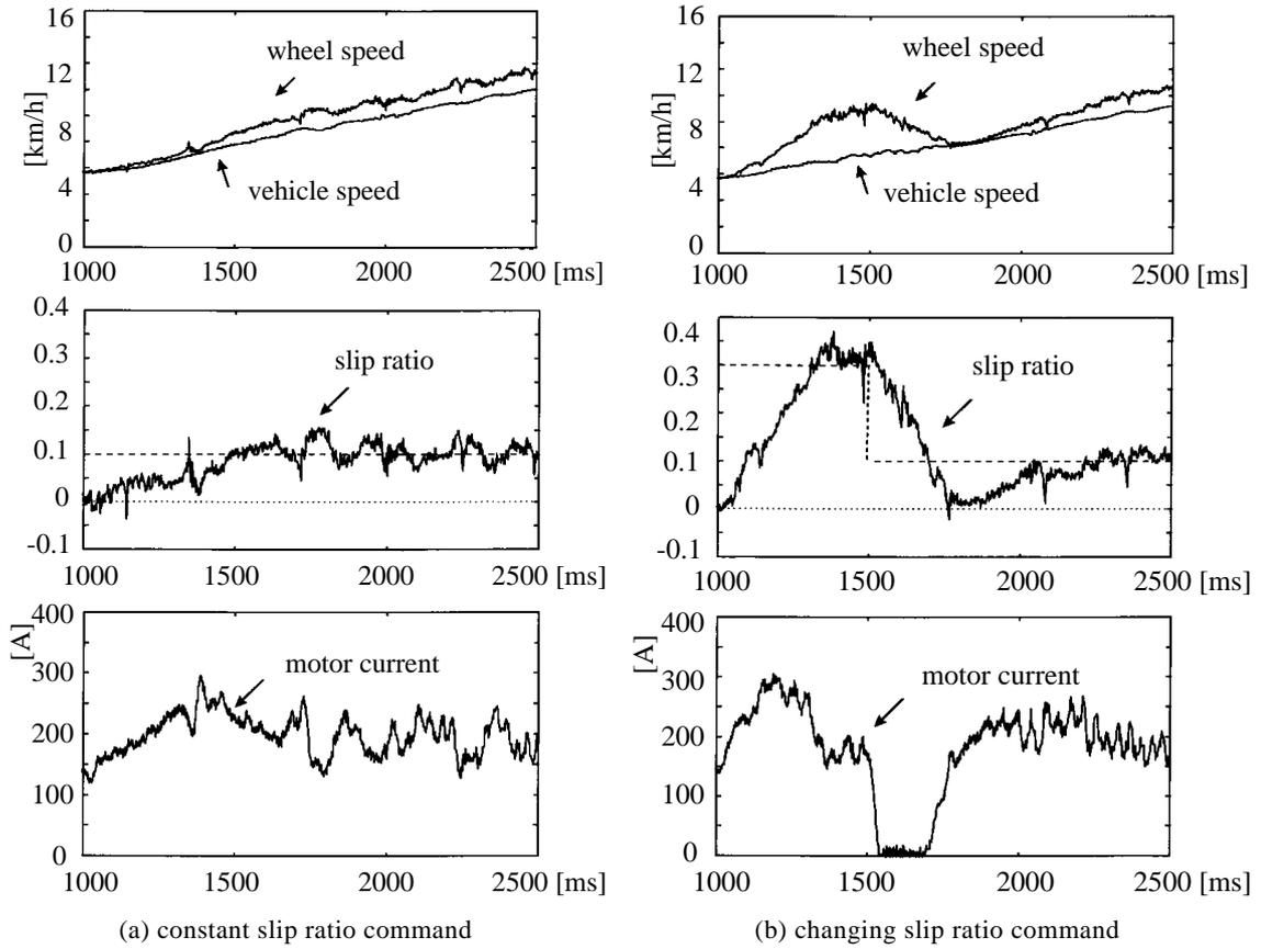
Fig.13. Experimental results of the slip ratio control
