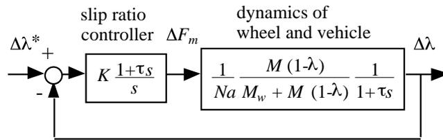
Fig.7. Slip ratio controller.
