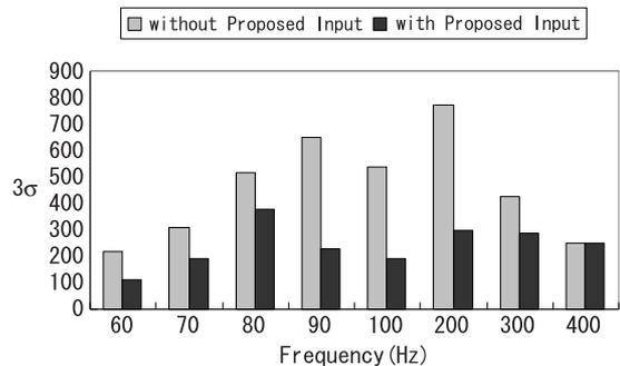
Fig.6: Comparison of  $3\sigma$  of Position Error Signal with/without Proposed Feedforward Input
