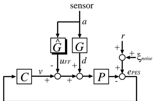
Fig.1: Block Diagram of Disturbance Rejection Control with Feedforward Input
