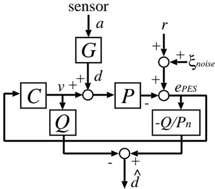
Fig.2: Block Diagram of Disturbance Observer to Estimate Disturbance
