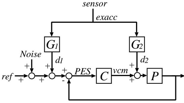
Fig.2: Block Diagram for Access Control of Hard Disk Drive System Under Vibration
