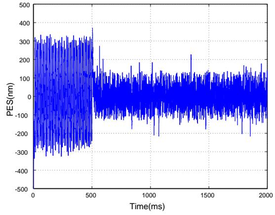
Fig.9: Time Series of PES under 100[Hz] vibration
