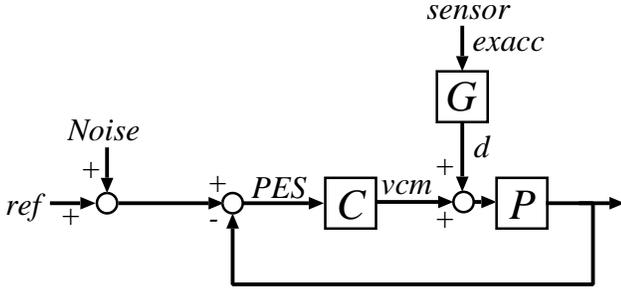
Fig.3: Transfer Characteristics from the Acceleration Sensor to Disturbance of the System
