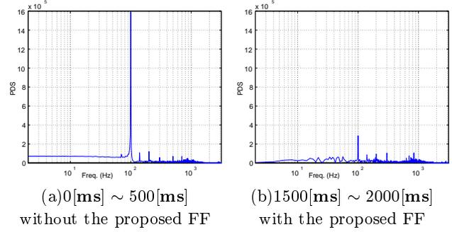
Fig.10: Characteristics of Fourier Transform about PES under 100[Hz] vibration
