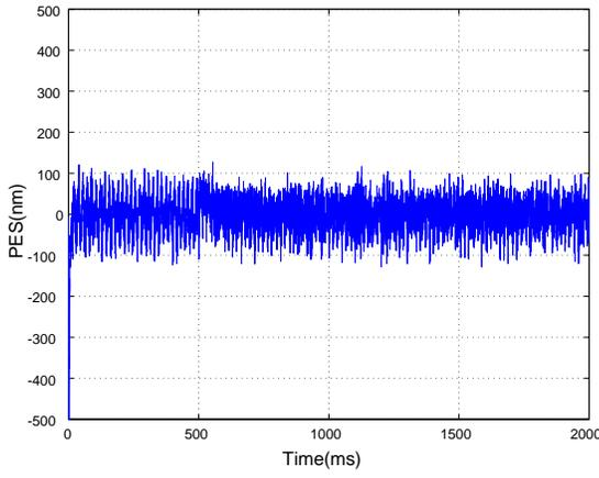
Fig.7: Time Series of PES under 60[Hz] vibration
