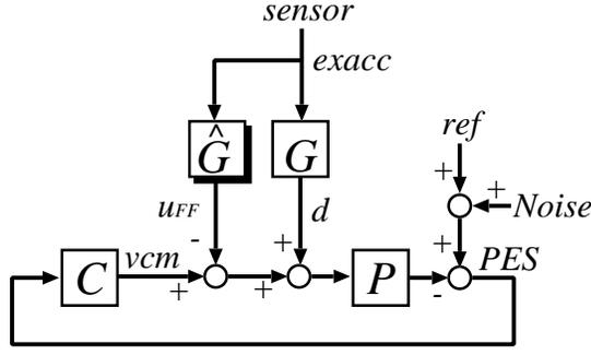
Fig.5: Block Diagram of Disturbance Rejection Control with Feedforward Input
