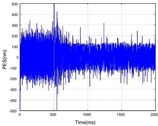
Fig.11: Time Series of PES under 300[Hz] vibration
