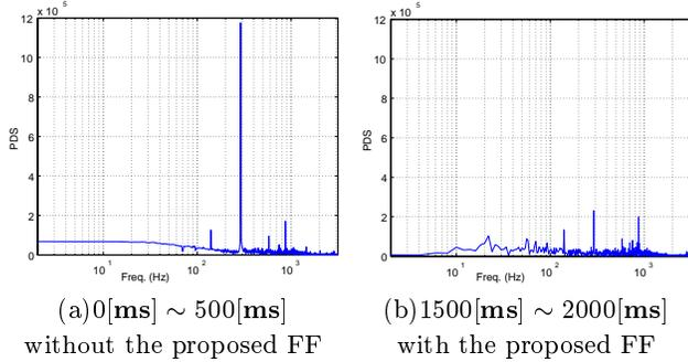
Fig.12: Characteristics of Fourier Transform about PES under 300[Hz] vibration
