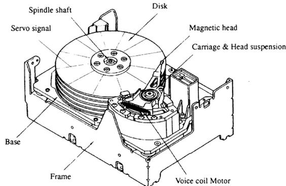
Fig.1: Overview of Hard Disk Drive System
