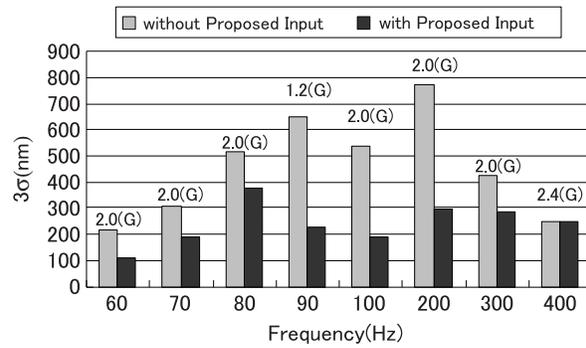
Fig.13: Comparison of  $3\sigma$  of PES with Proposed Input and without Proposed Input
