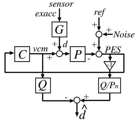
Fig.4: Block Diagram of the Disturbance Observer to Get the Estimated Disturbance
