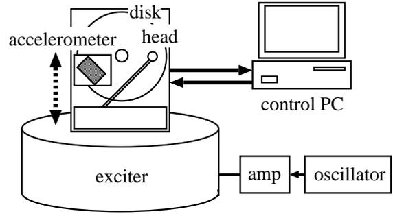
Fig.6: Configuration of Experimental System
