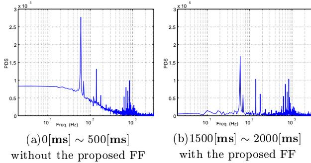
Fig.8: Characteristics of Fourier Transform about PES under 60[Hz] vibration
