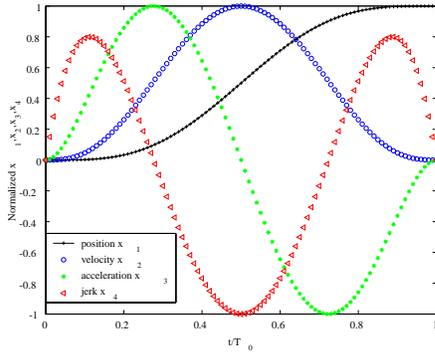
**Figure 3:** Normalized trajectory based on the equation (15) ~ (18)
