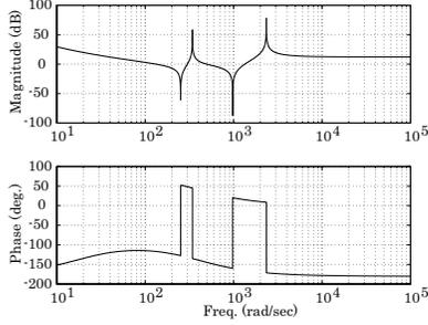
Fig. 8. Bode plot of  $G_l(s)$  in  $PID$  control
