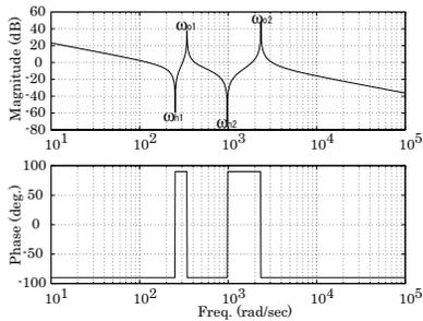
Fig. 4. Bode plot of the three-inertia model
