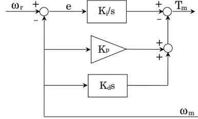
Fig. 6. Set-point-I  $PID$  controller
