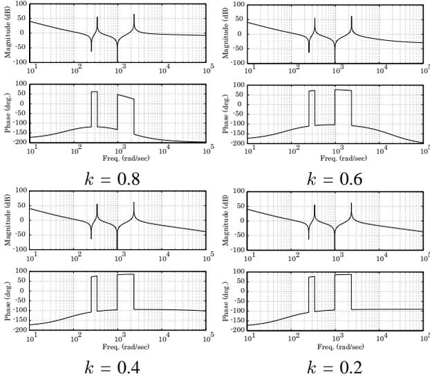
Fig. 9. Bode plots of  $G_l(s)$  in  $PID^k$  control
