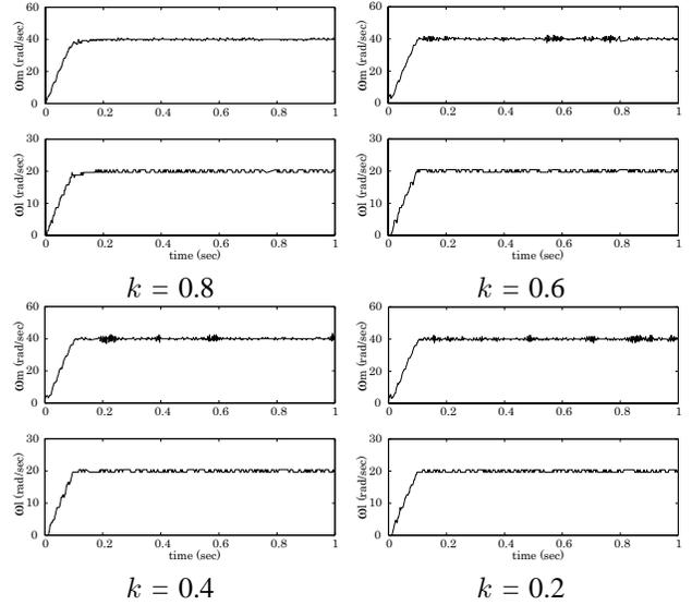
Fig. 15. Time responses of  $PID^k$  control ( $m = 5$ )
