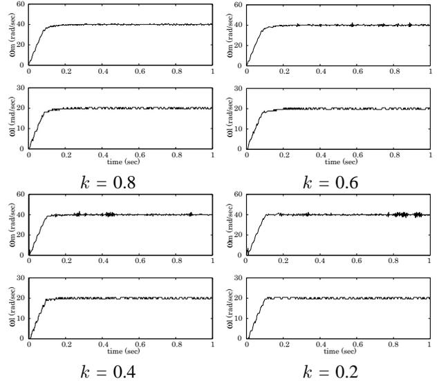
Fig. 16. Time responses of  $PID^k$  control ( $m = 100$ )
