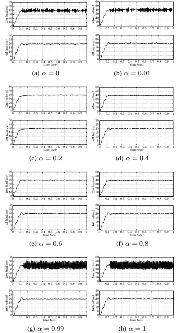
Figure 14. Time responses with fractional order  $\frac{1}{(Ts+1)^\alpha}$  filter
