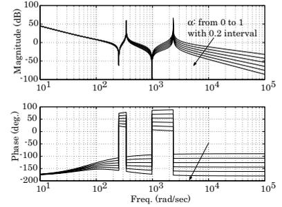
Figure 9. Bode plots of  $G_l(s)$  with fractional order low-pass filter
