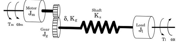
Figure 2. Torsional system's three-inertia model
