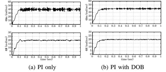
Figure 13. Improvement by introducing disturbance observer
