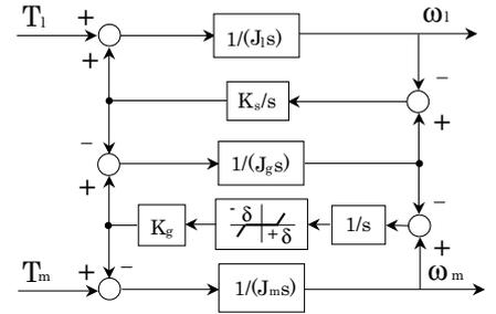
Figure 3. Block diagram of the three-inertia model
