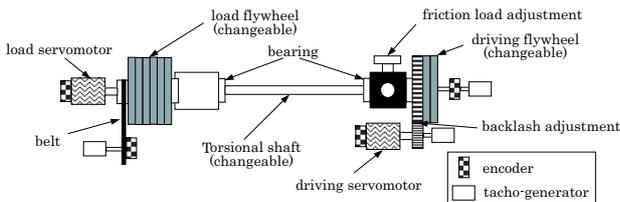
Figure 1. Experimental setup of torsional system
