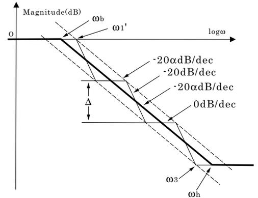
Figure 10. Broken-line approximation ( $N = 1$ )
