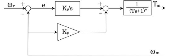
Figure 8. PI controller with fractional order low-pass filter
