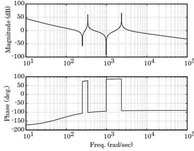
Figure 6. Bode plot of PI control system
