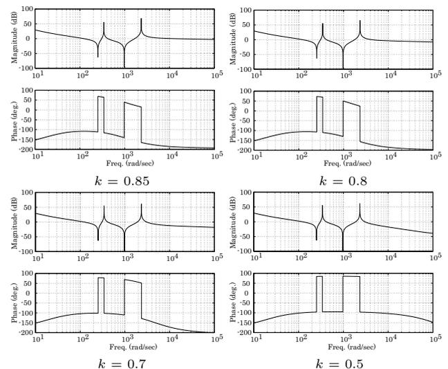
Fig. 9. Bode plots of  $G_l(s)$  in  $PID^k$  control
