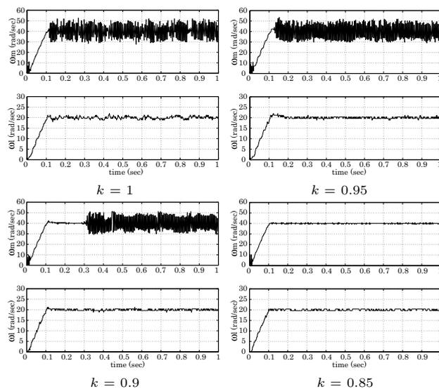
Fig. 16. Continuity of  $PID^k$  control's vibration suppression performance
