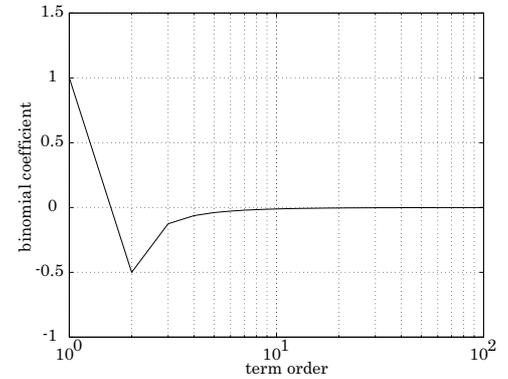
Fig. 12. Binomial coefficients value versus term order  $j$  when approximating  $D^{0.5}$
