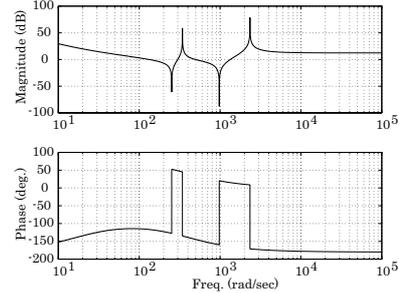
Fig. 8. Bode plot of  $G_l(s)$  in PID control
