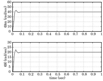
Fig. 7. Time responses of the integer order PID two-inertia system by simulation
