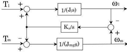
Fig. 5. Block diagram of the two-inertia model
