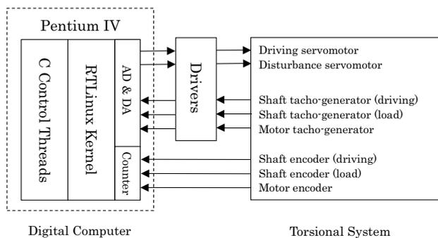
Fig. 13. Digital control system of the experimental setup
