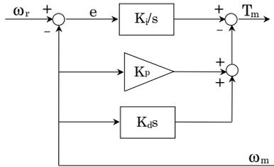
Fig. 6. Set-point-I PID controller
