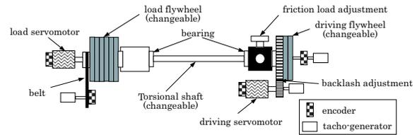
Figure 1. Experimental setup of torsional system
