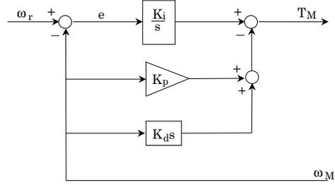
Figure 5. Set-point-I *PID* controller
