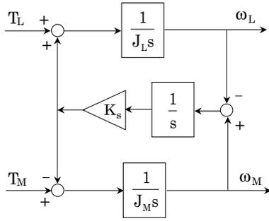
Figure 3. Block diagram of two-inertia system
