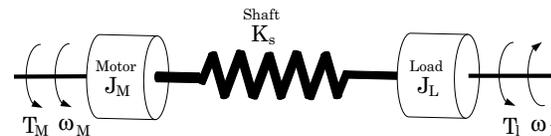
Figure 2. Two-inertia system model
