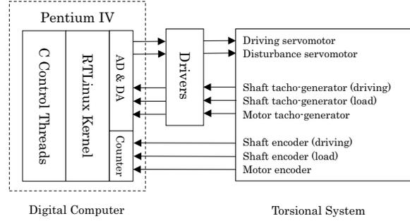
Figure 13. Digital control system of the experimental setup
