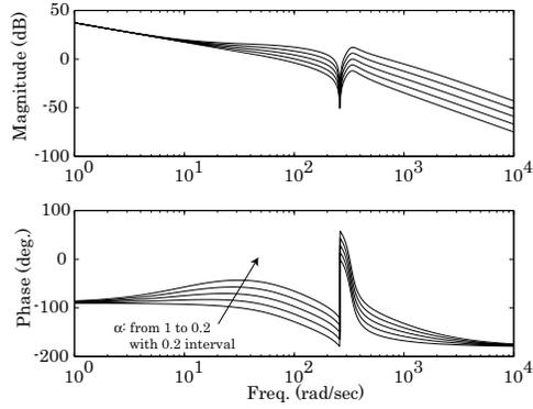
Figure 8. Bode plots of fractional order  $PI^\alpha D$  control systems
