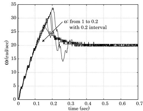
Figure 15. Step responses of load side with input torque saturation
