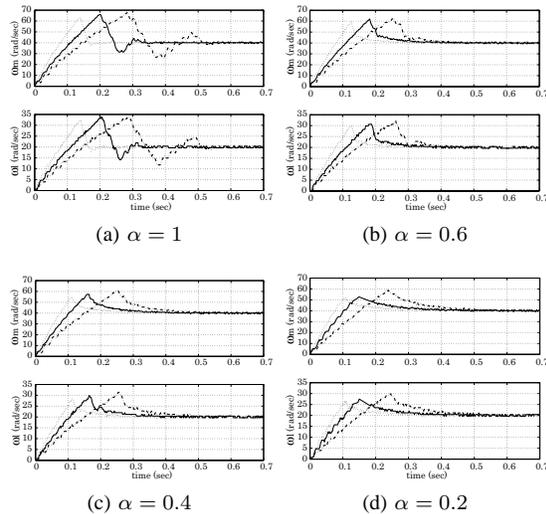
Figure 16. Step responses of  $PI^\alpha D$  system with load inertia variation. (solid line: nominal case; dotted line:  $0.3J_l$ ; broken line:  $1.7J_l$ )
