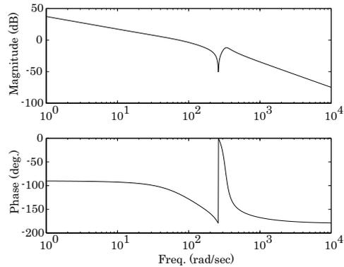
Figure 7. Bode plot of designed integer order *PID* control system
