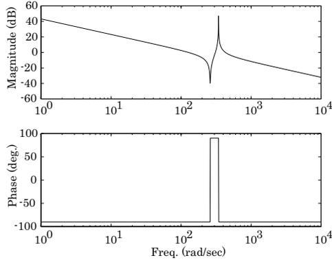
Figure 4. Bode plot of the two-mass plant
