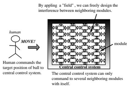
**Fig. 11.** Combined control of central / autonomous decentralized algorithms.
