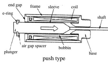
**Fig. 6.** Configuration of the solenoid plunger.
