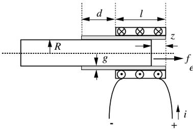
Fig. 9. Electromagnetic model of the solenoid plunger. Electromagnetic force generated in this solenoid plunger is calculated by using this simple model.
