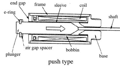
Fig. 10. Configuration of the solenoid plunger.
