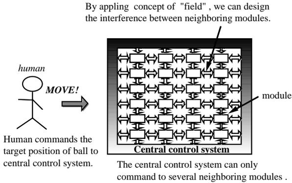
Fig. 2. Combined control of central / autonomous decentralized algorithms.
