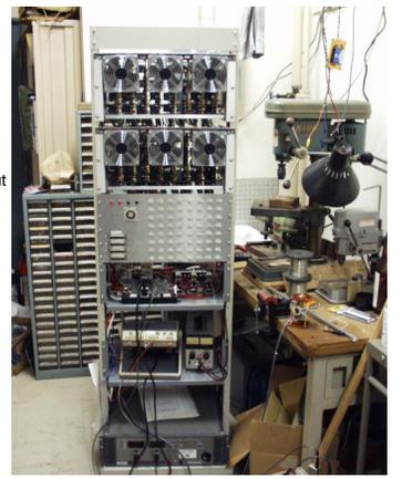
Fig. 6. Overview of the experimental setup including 64 controllers and main power supply.
