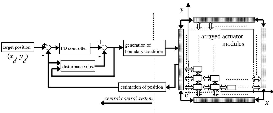
Fig. 3. Block diagram based on object position feedback control with object position estimation
