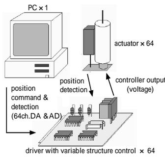
Fig. 5. Outline of the experimental setup consisting of 64 variable structure controllers, 64 linear drive actuators and "one" PC.
