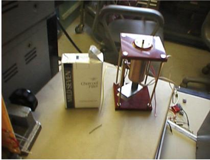
Fig. 8. The real world actuator module consisting of solenoid plunger. We can easily see attached position sensor. This position sensor is putted to use position signal in feedback controller.
