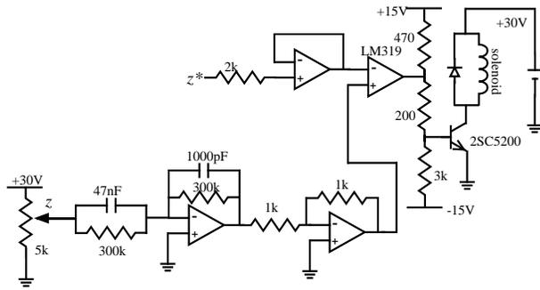
Fig. 12. Analog circuit of the variable structure controller. This variable structure controller actually used in the experiment. 64 sets of this analog circuit are prepared for realization of magic carpet. This circuit is very simple and adopted for position controller.
