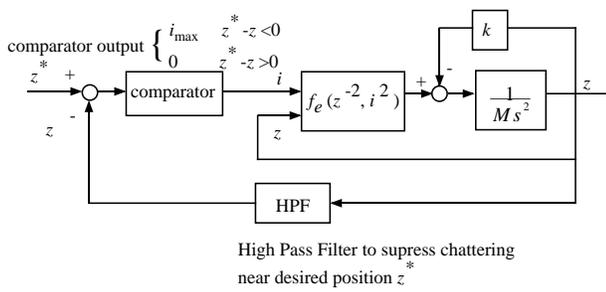
Fig. 11. Control system of solenoid plunger with variable structure controller.
