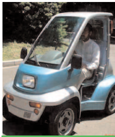
Fig.5. Comus CV (driven only by ultra-capacitors)
