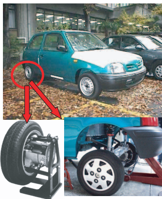
Fig. 1. "UOT March II" and in-wheel motors.
