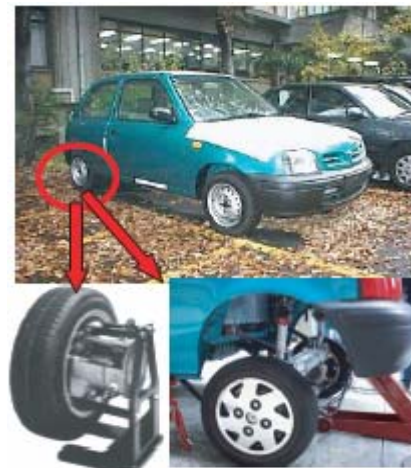
Fig. 1 “UOT March II” and its in-wheel motors
