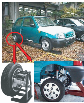
Fig. 1. "UOT March II" and in-wheel motors.
