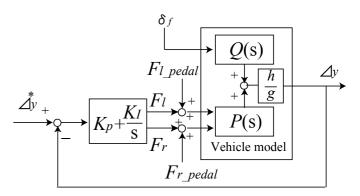
Fig. 6 NFS control diagram
