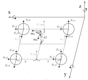
Fig. 4 Normal force on each tire
