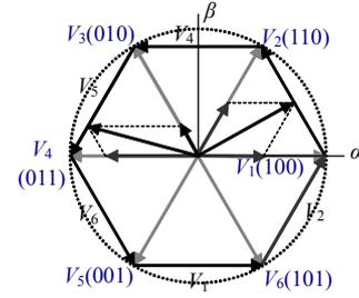
Fig.2 The discretized voltage vectors and their synthesis
