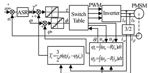
Fig.5 The DTC control system for PMSM
