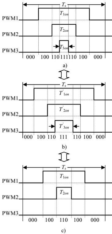
Fig.3 The correction of digital SPWM waves
