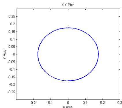
Fig.6 The simulation curve of stator flux
