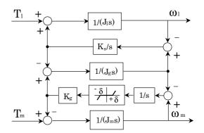
Fig. 3. Block diagram of the three-inertia model
