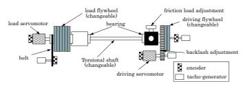
Fig. 1. Experimental setup of torsional system
