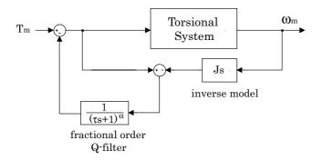
Fig. 10. Disturbance observer with fractional order Q-filter
