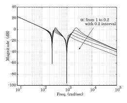
Fig. 11. Gain plot from  $T_m$  to  $\omega_m$  with different  $\alpha$
