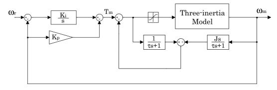
Fig. 7. Block diagram for simulation with three-inertia model
