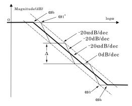
Fig. 12. An example of broken-line approximation (N = 3)
