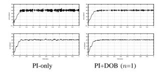
Fig. 16. Comparison of PI-only control and PI+DOB control
