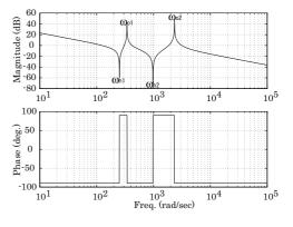
Fig. 4. Bode plot of the three-inertia model
