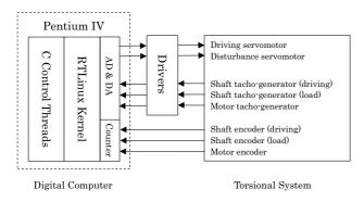
Fig. 14. Digital control system of experimental torsional system
