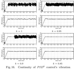
Fig. 16. Continuity of  $PID^{\kappa}$  control's vibration suppression performance
