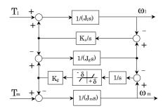
Fig. 3. Block diagram of the three-inertia model
