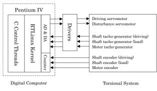
Fig. 13. Digital control system of the experimental setup
