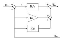
Fig. 6. Set-point-I PID controller
