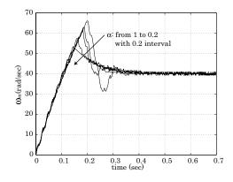
Figure 14. Step responses of driving motor with input torque saturation
