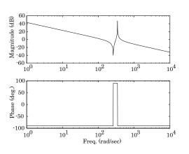
Figure 4. Bode plot of the two-mass plant
