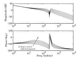
Figure 8. Bode plots of fractional order  $PI^{\alpha}D$  control systems
