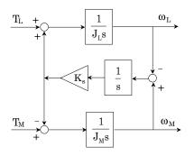
Figure 3. Block diagram of two-inertia system
