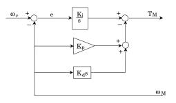
Figure 5. Set-point-I PID controller
