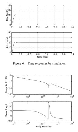
Figure 7. Bode plot of designed integer order PID control system
