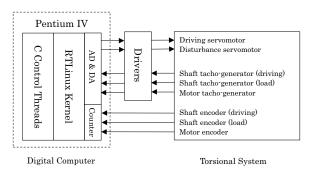
Figure 13. Digital control system of the experimental setup
