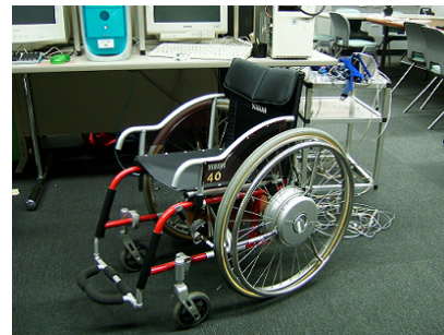
Fig. 1. Power-assisted wheelchair as an experimental tool (YAMAHA JW II)
