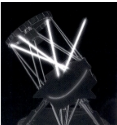
Fig. 3: Overview (2) of astronomical telescope "subaru". It is difficult to condense the ray of right because of distortion of the mirror by self weight.
