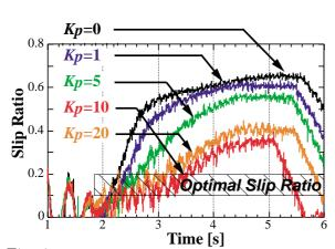
Fig. 8: Effect of wheel velocity control for skid prevention with  $\tau=0.1$ [s] (Experimental results.)  $K_p^*$  of Eq. (16) is 4.52 for this vehicle.
