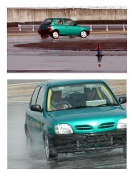
Fig. 11: Photo of turning experiments with 4Wmotored EV "UOT Electric March II" (Fig. 12-13).
