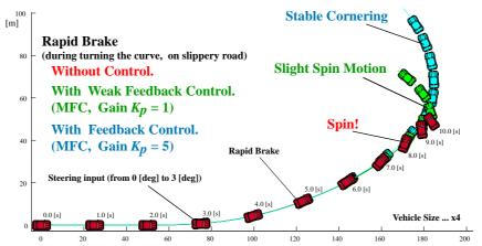
Fig. 10: Stabilizing effect with "controlled four wheels" is visualized with vehicle's trajectory [6].
