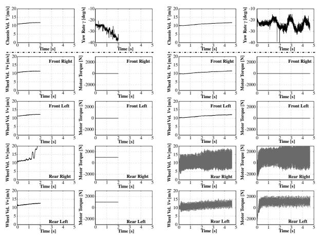
Fig. 12: Unstable turning with sudden acceleration torque on rear wheels. Vehicle made steady turning before torque inputs.
