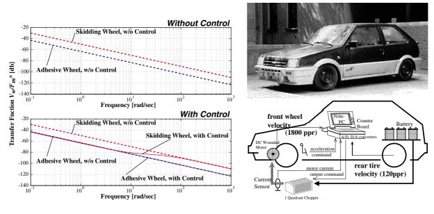
Fig. 6: Bode diagram of  $V_w/F_m^*$ .
