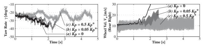
Figure 14: Comparison of vehicle motion: (a) without feedback controller, (b) with weak feedback controller, (c) and adequate feedback controller.  $K_p^*$  is 45.2 for this vehicle.  $\tau$  in the controller was 0.1 [s].
