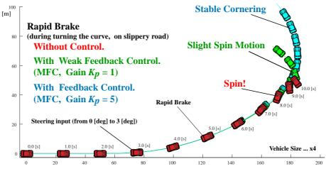
Figure 11: Stabilizing effect with "controlled four wheels" is visualized with vehicle's trajectory [6].
