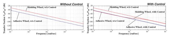
Figure 8: Bode diagram of  $V_w/F_m^*$ .  $K_p = K_p^* = \frac{M+M_w}{M_w}$ .  $\tau = 0.1[sec]$ .
