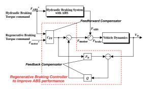
Figure 16: "H-ABS", cooperative ABS with both electric and hydraulic torque.
