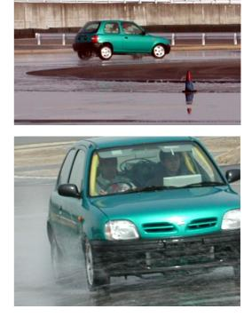
Figure 4: Photo of turning experiments with 4Wmotored EV "UOT Electric March II" (Fig. 12-13).
