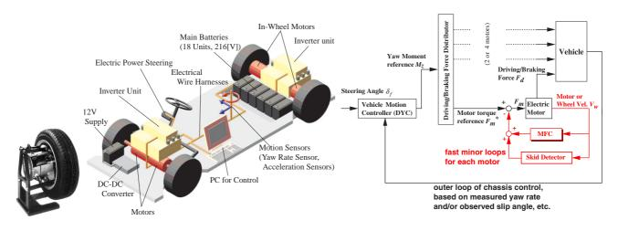
Figure 1: In-wheel motor (left) and our new EV with four in-wheel motors. (right)
