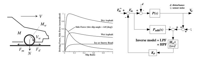
Figure 5: One wheel model. Figure 6: Typical  $\mu - \lambda$  curve. Figure 7: Proposed feedback controller.
