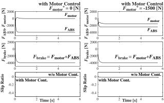
Fig. 16. Simulation results with adhesive road.
