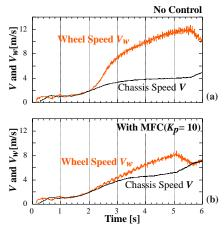
Fig. 8. Wheel and chassis velocity with and without MFC.
