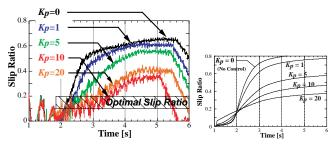
Fig. 7. MFC effect for skid prevention with  $\tau$ =0.1[s] (Left fig.: Experimental results / Right fig.: Simulation results)
