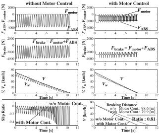
Fig. 17. Simulation results with slippery road. (  $F_{\rm motor}^* =$  -1500 [N] )
