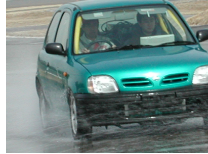
Figure 11: Photo of turning experiments with 4W-motored EV “UOT Electric March II”
