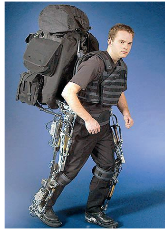
Berkeley Lower Extremity Exoskeleton
