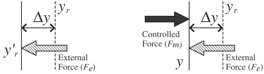
a) Reference position ( y' ) is changed according to the external force ( F_e ). b) Motor torque ( F_m ) is changed according to the displacement ( \Delta y ).
