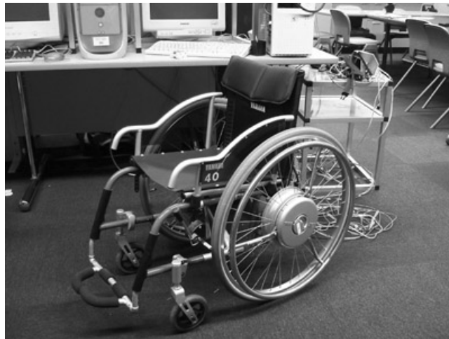
Figure 1.6: Power-assisted wheelchair as an example of power assist device(YAMAHA JW II)
