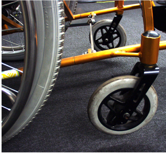
Figure 4.15: Casters as front wheels of a wheelchair
