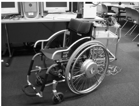
Figure 1: Power-assisted Wheelchair as an Example of Power Assistance Tools (YAMAHA JW II)
