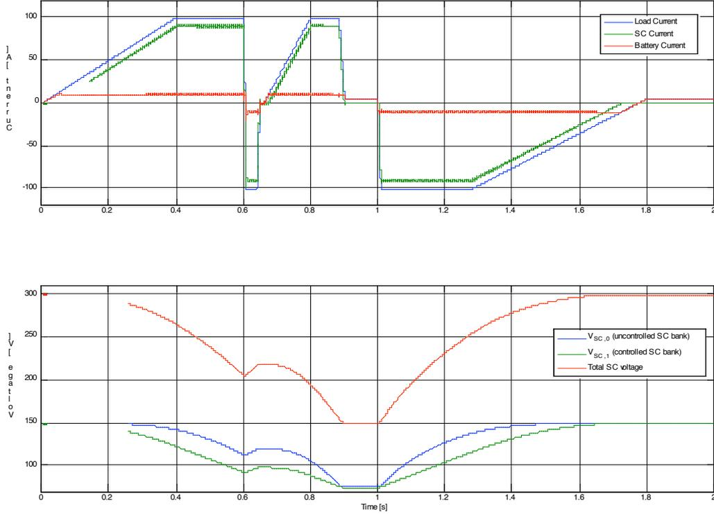
Fig. 4 – Simulation of charge/discharge cycle with the proposed Half-Controlled Converter.
