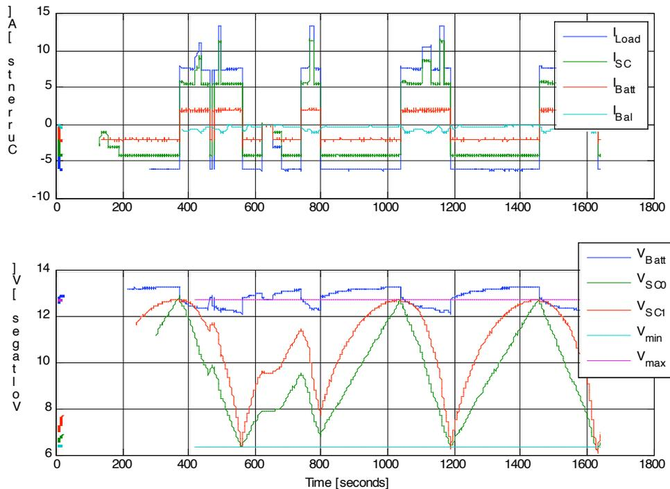
Fig. 6 – Experimental Results; Charge/Discharge cycles with arbitrary load current waveform.
