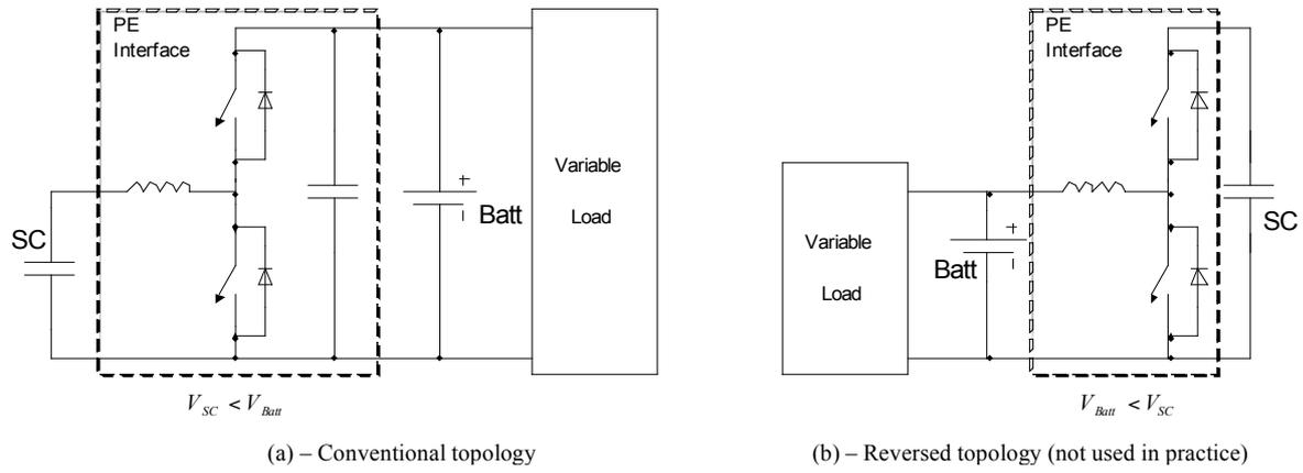
Fig.2 – Power Electronics interfaces based on Half-Bridge topology
