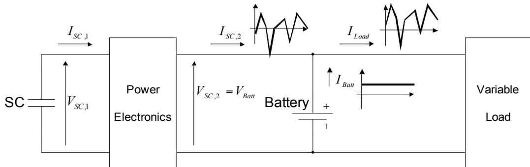
Fig.1 – Basic SC-Battery Mixed System with Power Electronics Interface
