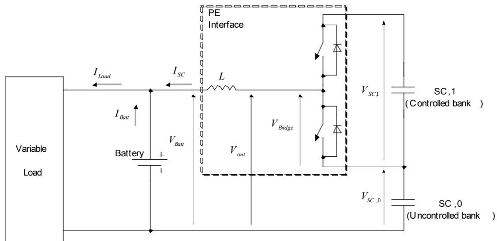
Fig. 3 – Half Controlled Cascaded Converter
