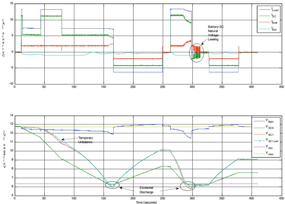
Fig. 7 – Experimental Results; Quick Discharge and natural recovery after excessive discharge.
