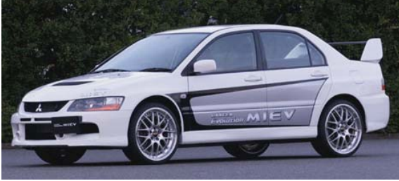
Fig. 2. LANCER EVO-MIEV (Test EV made by Mitsubishi Motors. It has four in-wheel-motors, which can be controlled independently. lithium-ion batteries under the floor provide the power for the four wheel drive system.
