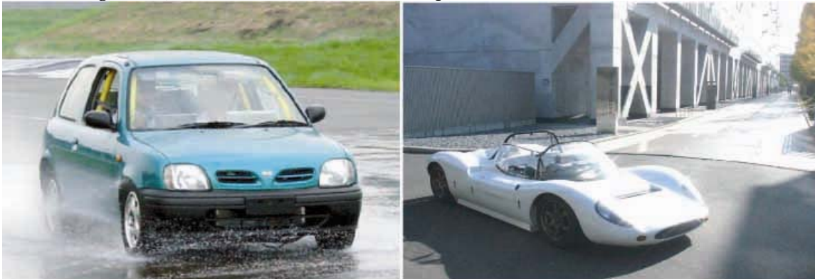
4WD in-wheel motored EV named "UOT March II"
