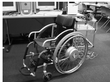
Fig. 1. Power assist wheelchair as an experimental setup (YAMAHA JW II)
