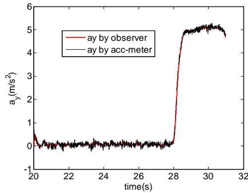
b) Nonlinear area (driver steering angle=90° , v=60Km/h)
