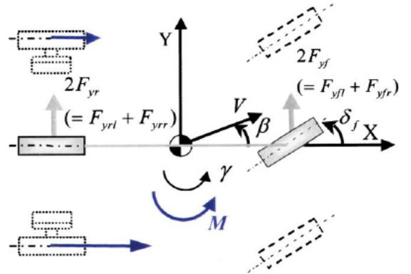
Fig.2 two-freedom vehicle model for observer design
