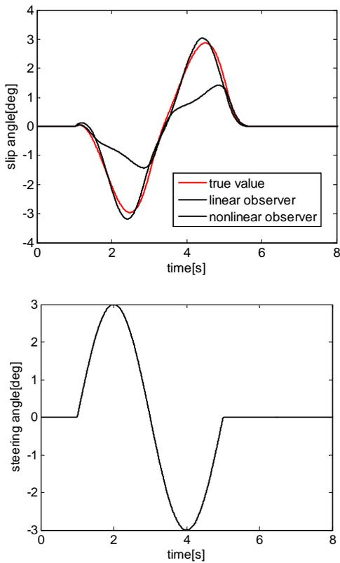
Fig.4 Lane change maneuver simulation results of slip angle observer
