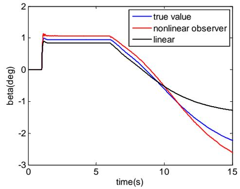
Fig.5 simulation results of slip angle observer (Vehicle accelerates with constant  $\delta_f = 3^\circ$ )
