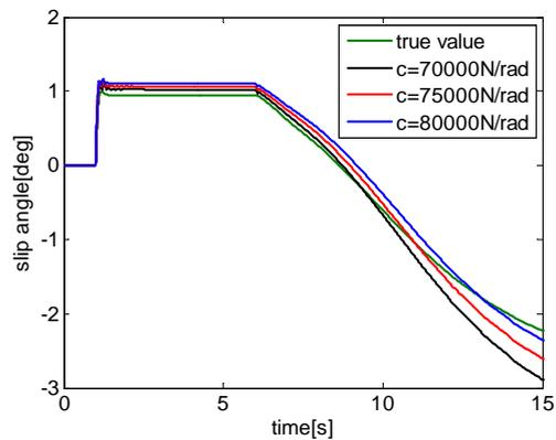
Fig.7 simulation results with different stiffness values
