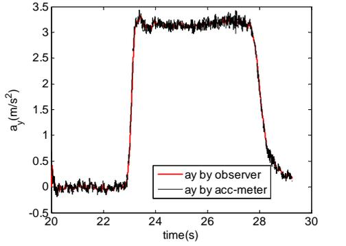
a) Linear area (driver steering angle=90° , v=40Km/h)
