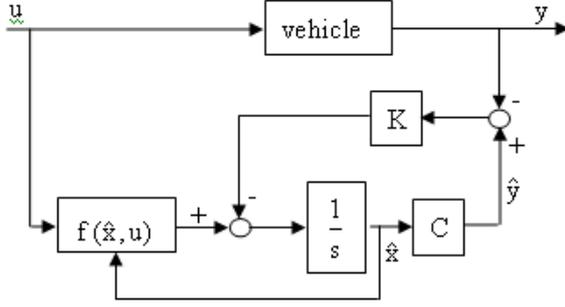
Fig. 1  $\beta$  observer with nonlinear tire model
